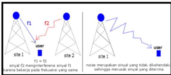
Figure 6. Difference between Interference and Noise
