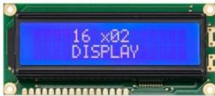
Fig 10. Physical form of LCD 16x2 [11]
